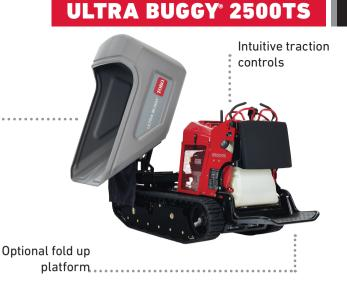
Built on the trusted tracked Ultra Buggy frame, the swivel buggy gives you a 180 degree dump radius, plus:
