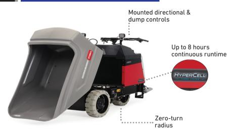
Toro's electric Ultra Buggy is the next evolution in material handling. Electric power eliminates engine exhaust emissions, and the thick, polyethylene tub handles all types of material.
